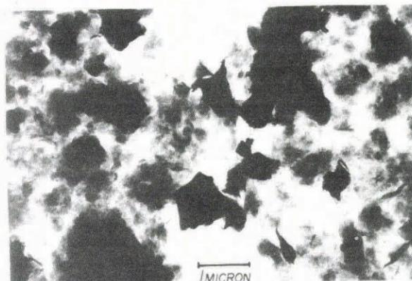
Fig.1. Photoelectron micrograph of activated clay particles.
