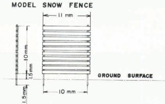
Fig.4. Model snow fence on the scale of 1/300.
