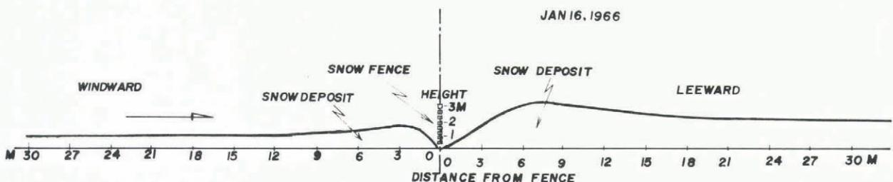
Fig.9. Cross section of a prototype snowdrift formed around the prototype snow fence measured by T. Uchiya (1967) in Teshio, Hokkaido, in January 1966.
