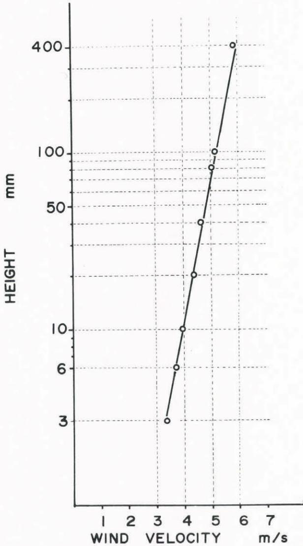
Fig.5. Wind profile used in the modeling of a snowdrift.
