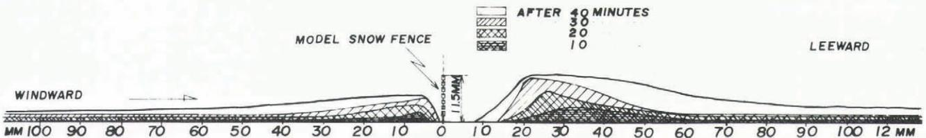
Fig.8. Change in the cross section of the model snowdrift formed around the model snow fence as a function of time.
