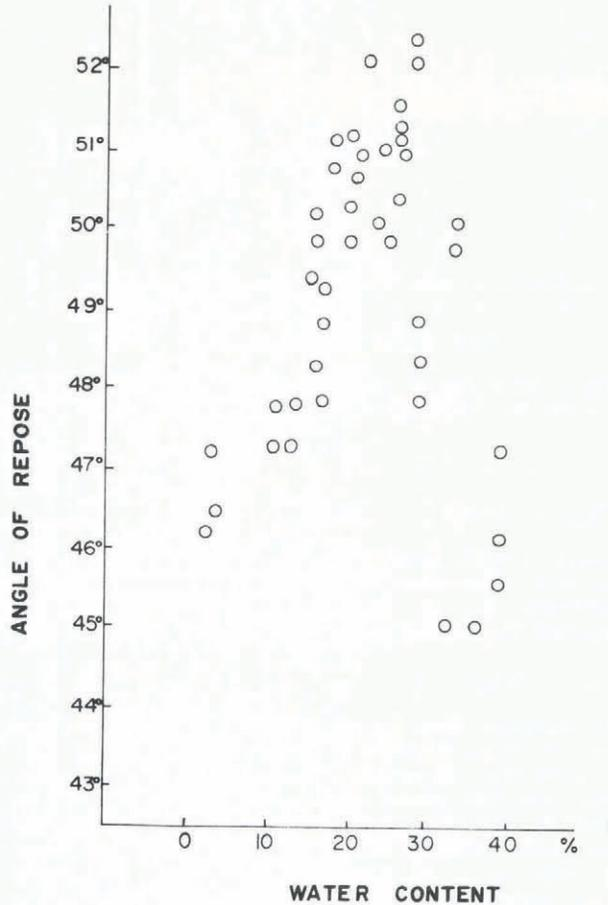
Fig.2. Angle of repose of activated clay particles versus their water contents.
