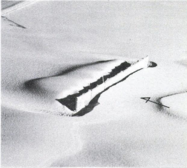
Fig.7. Model snowdrift formed around the model snow fence.
