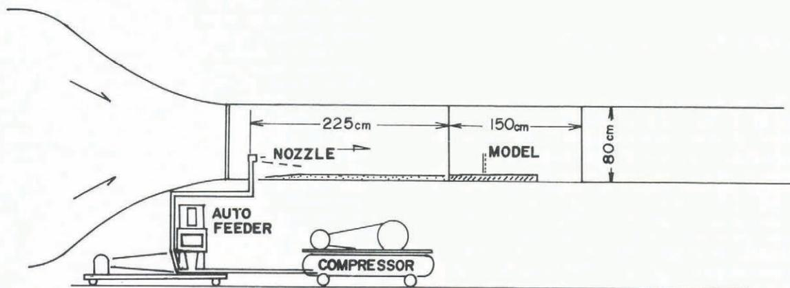
Fig.3. Testing section of the experimental wind tunnel used.
