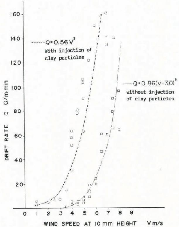
Fig.6. Drift rate of activated clay particles versus wind speed at a height of 1 cm in the wind tunnel.
