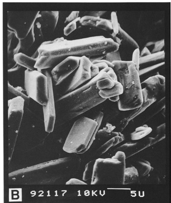
Figure 2. SEM microphotographs of A) Ba-bearing clinoptilolite (404.5 m) and B) Ba-free clinoptilolite (676.7 m).
