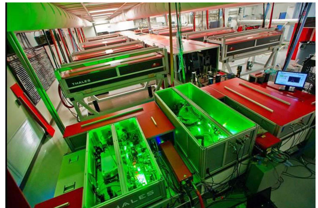
Figure 7. The BELLA laser facility, the world's first 1 Hz petawatt laser (picture courtesy of Lawrence Berkeley National Laboratory).
