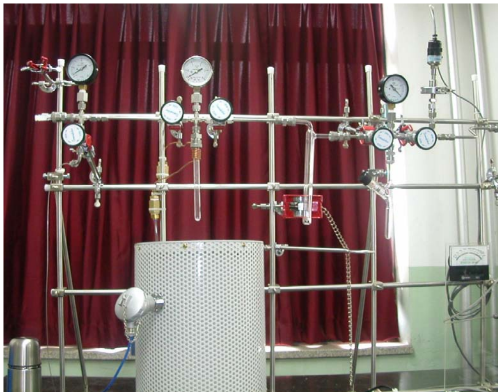
Figure 2 Photograph of the present combustion system for liquid and gas samples
