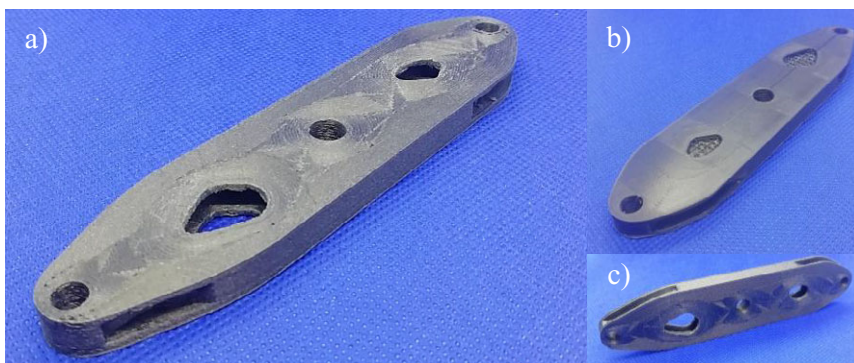
Figure 19. Printed scissor arm. (a) Surface concentric without ‘ironing’. (b) Surface ‘ironed’ and including lattice. (c) Upright view.
