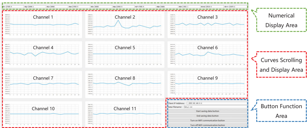
Figure 5. GUI with data display and save function developed based on Qt framework.
