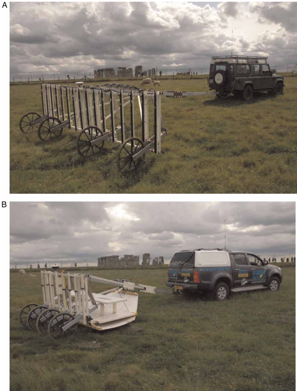
Figure 2. Vehicle-towed geophysical survey equipment used in the 2011 surveys at Stonehenge. (A) Sixteen channel magnetometer. (B) AMOS electromagnetic system. Photographs: Timothy Darvill.
