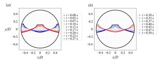
Figure 16. Wave profile 0.5 fill level,  $\gamma = 2$  mm, f = 3.785 Hz: (a) increasing wave elevation through the FSC; (b) decreasing wave elevation through the FSC.
