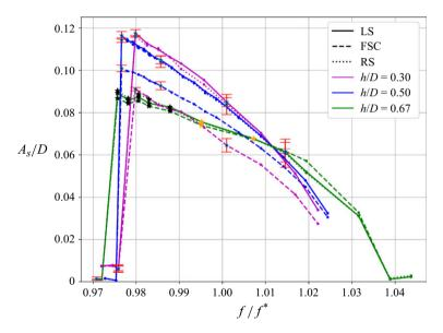
Figure 15. Steady-state sloshing wave amplitude (FSC, RS and LS) expressed against excitation frequency for three different fill levels, h/D = (0.3, 0.5, 0.67). Black markers indicate wave breaking, orange markers indicate period tripling, all other markers are non-monochromatic waves.
