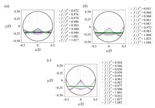
Figure 13. The 0.3 fill level maximum and minimum free surface centre elevation, for all tested frequencies: (a) forcing amplitude,  $\gamma = 2$  mm; (b) forcing amplitude,  $\gamma = 3$  mm; (c) forcing amplitude,  $\gamma = 4$  mm.
