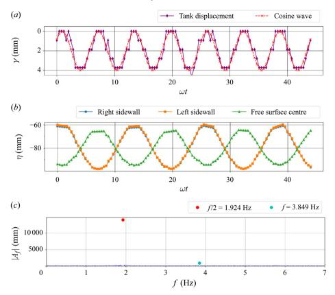
Figure 10. The 0.3 fill level, forcing frequency  $f = 3.850 \,\mathrm{Hz}$  ( $f/f^* = 1.016$ ) and forcing amplitude  $\gamma = 2 \,\mathrm{mm}$ : (a) tank displacement; (b) steady-state sloshing wave amplitude of the (FSC, RS and LS); (c) DFT of sloshing wave amplitude at the FSC.
