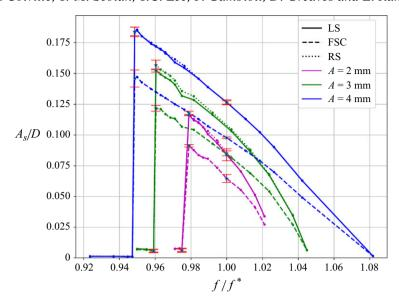
Figure 11. Steady-state sloshing wave amplitude,  $A_s$  (FSC, RS and LS) expressed against excitation frequency for different forcing amplitudes and a constant fill level h/D = 0.3.
