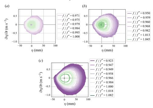
Figure 12. Velocity phase plane diagrams (0.3 fill level) where  $\eta$  is the FSC elevation, f is the forcing frequency and  $f_2$  is the first symmetric linear wave frequency: (a) forcing amplitude  $\gamma = 2$  mm; (b) forcing amplitude  $\gamma = 3$  mm; (c) forcing amplitude  $\gamma = 4$  mm.
