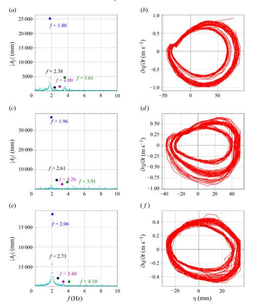
Figure 17. Frequency domain and phase plane tripling: (a) DFT of h/D=0.3, f=3.595 Hz and  $\gamma=4$  mm; (b) phase plane of h/D=0.3, f=3.595 Hz and  $\gamma=4$  mm; (c) DFT of h/D=0.5, f=3.920 Hz and  $\gamma=4$  mm; (d) phase plane of h/D=0.5, f=3.920 Hz and  $\gamma=4$  mm; (e) DFT of h/D=0.67, f=4.05 Hz and  $\gamma=2$  mm; (f) phase plane plot of h/D=0.67, f=4.05 Hz and  $\gamma=2$  mm.
