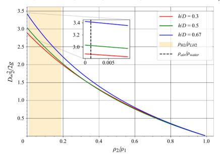
Figure 5. Variation of first symmetric mode in terms of density ratio. The density ratio of air—water  $\rho_{air}/\rho_{water}$  and the maximum and minimum values of the density ratio range considered in figure 4 are highlighted.
