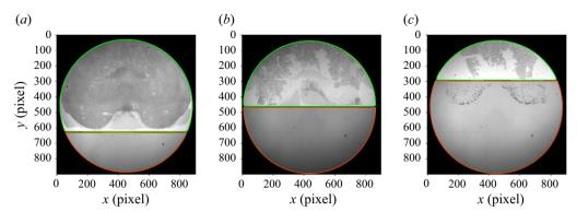
Figure 8. Static fluid reference cases with extracted liquid (orange) and gas (green) phase overlaid, respectively. (a) h/D = 0.3; (b) h/D = 0.5; (c) h/D = 0.67.
