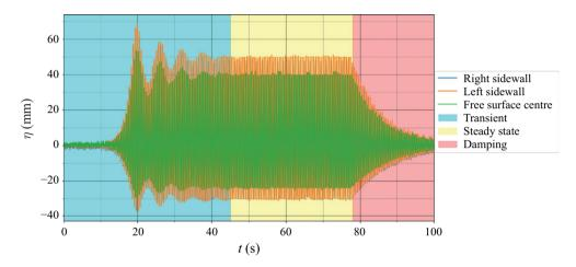
Figure 9. Free surface elevation ( $\eta$ ) against time (t) showing transient, steady-state and damping regimes for the fundamental symmetric mode anti-nodes; 0.3 fill level,  $\gamma = 4$  mm and f = 3.86 Hz.
