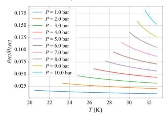
Figure 4. Density ratio range in a sub cooled LH2 fuel tank (Bell *et al.* 2014). Liquid hydrogen density,  $\rho_{LH2}$ , is 73.2 kg m<sup>-3</sup> assuming the constant temperature T = 20 K. The gas density,  $\rho_{H2}$ , is considered in the pressure range of P = 1 - 10 bar at temperatures between the hydrogen triple and critical temperatures  $T_t = 13.97$  K and  $T_c = 33.15$  K, respectively.
