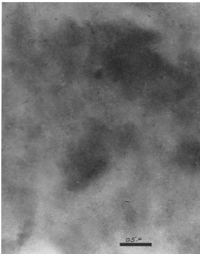
PLATE 11. Mullite crystallization in Wyoming montmorillonite at 1000°C.
