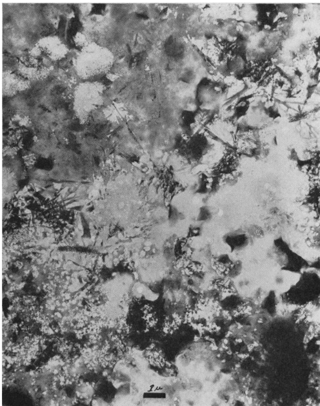
PLATE 10. Cristobalite crystals in Cheto montmorillonite after 35 min at 1200°C.
