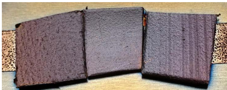
Figure 1: Au/Pd coated HDPE bottles, showing differences in surface texture. From left to right: jug, tan bottle, and flame treated.
