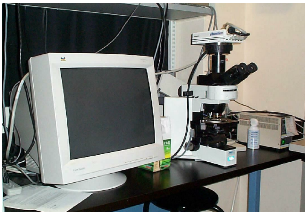
FIG. 2. Fluorescence Computerized Image Analysis system with motorized stage and cooled CCD camera.
