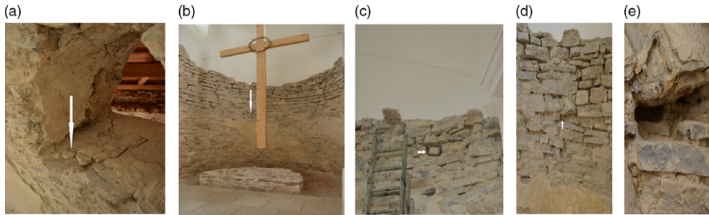
Figure 6 Examples of sampling sites in the Rotunda interior: wood sampling point W6 (1041) in the pre-Romanesque window (a); charcoal C2 (1042) point at the apse closing (b); mortar M1 (1049) point at the northeastern part of the nave (c); mortar M2 (1045) point at the eastern part of the apse wall, and in detail (e).
