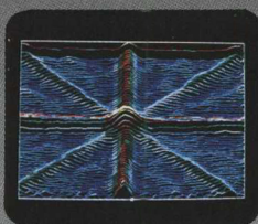
Three dimensional display of angle resolved channeling.
