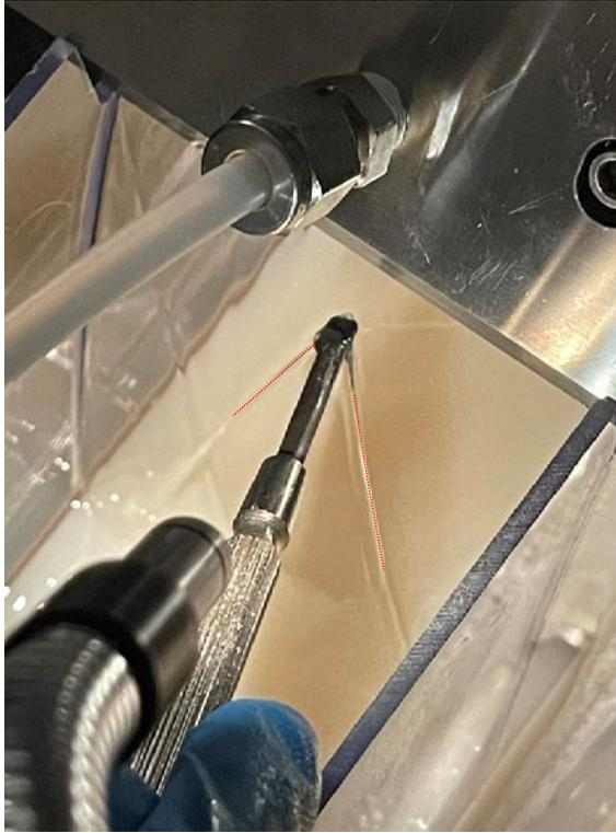
Figure 7. Standing waves demonstrating that a volumetric flow rate per unit length of  $Q^* = 3.7 \text{ cm}^2 \text{ s}^{-1}$  leads to  $We_l > 1$  everywhere in the curtain (see also figure 4). The standing waves have been enhanced with a red line to facilitate the visualization.
