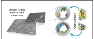
The bioinspired hybrid membrane shows the orientation of Gramicidine A inside the cylindrical nanopores. Reproduced with permission from Nano Lett. 11 (2)(2011), DOI: 10.1021/ nl103841m; p. 712. © 2011 American Chemical Society.
