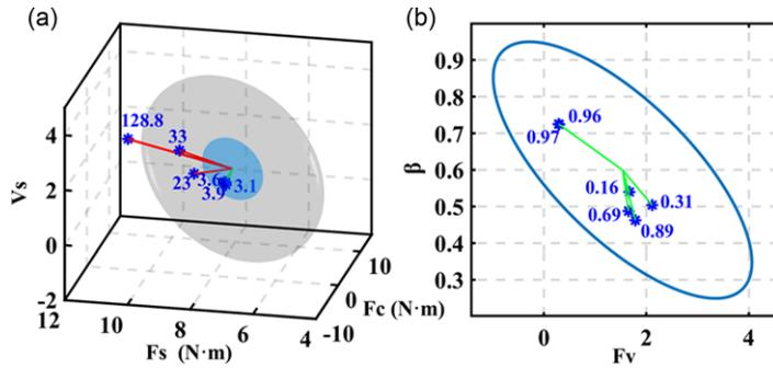
**Figure 14.** The confidence regions for joint 3. (a) The blue and gray regions are the 2- and 6-standard-deviation ellipsoids for velocity-weakening parameters. (b) The 2-standard-deviation ellipse for velocity-strengthening parameters.
