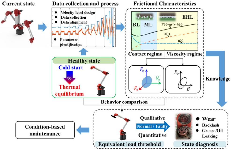
**Figure 2.** Framework of the proposed diagnosis approach for the joint of a robot manipulator. BL refers to boundary lubrication, which is mainly related to the interaction between the micro-asperities on the contacting surface. ML refers to mixed lubrication, where the interaction between micro-asperities coexists with the effects of a lubricating film. EHL refers to elastic hydrodynamic lubrication, which reaches a total separation of the surfaces by the lubricant.
