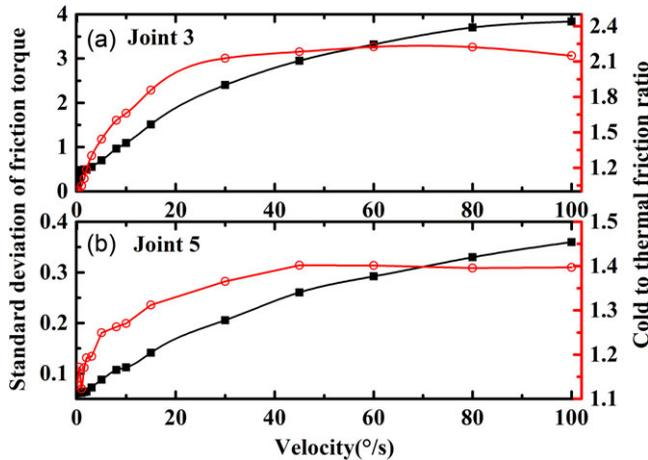
**Figure 11.** The standard deviation of friction torque at different operating times and temperatures (black solid line with rectangle symbols, left Y-axis). The cold-to-thermal friction ratio at different velocity levels (red solid line with circle symbols, right Y-axis).
