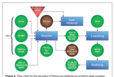
of Umicore). The blue rectangles indicate the steps in the process, whereas the green and brown circles represent material inputs and outputs, respectively. The red triangle shows an energy input of 800 MJ.
