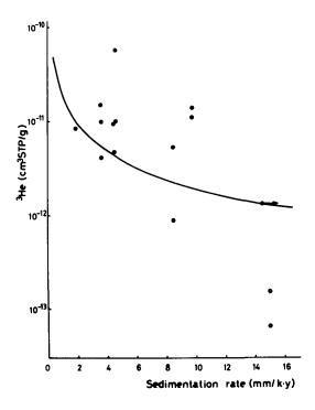
Figure 2.  $^3\text{He}$  content is plotted against sedimentation rate. Two hollow circles indicate the Atlantic DSDP samples which are of Cretaceous age. The Pacific samples (solid circles) show approximate inverse relation between  $^3\text{He}$  content and sedimentation rate. The curve is constructed by assuming uniform fallout rate (2000 tons/y) of cosmic dust ( $^4\text{He} = 0.1 \text{ cm}^3\text{STP/g}, \, ^3\text{He}/^4\text{He} = 4 \times 10^{-4}$ ).
