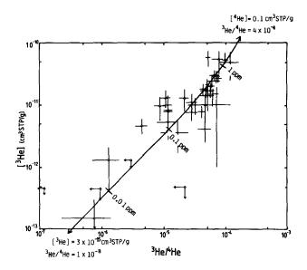
Figure 1.  $^3$ He content in sediments is plotted against  $^3$ He/ $^4$ He ratio. The curve indicates a mixing curve between He in the cosmic dust ( $^4$ He = 0.1 cm $^3$ STP/g,  $^3$ He/ $^4$ He = 4 x 10 $^{-4}$ ) and in the sediments ( $^3$ He = 3 x 10 $^{-15}$  cm $^3$ STP/g,  $^3$ He/ $^4$ He = 10 $^{-8}$ ). Numerical figures shown on the curve indicate the degree of the contamination (in ppm) of the cosmic dust in sediments.
