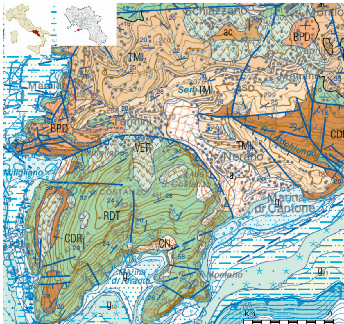
Figure 2. Geological map of the Termini-Nerano area (Iannace et al., 2015, modified). TM_1 = Termini sandstone, CDR = Calcareniti di Reconnone, RDT = Calcari a Radiolitidi, a_1 = landslide deposits, BOD = Breccia di Punta del Capo, VEF_1 = Vesuvian Flegrean Synthem.
