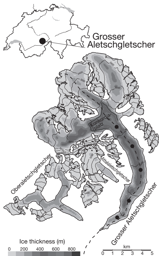
Fig. 1. Overview map of Grosser Aletschgletscher and smaller glaciers in the drainage basin. Glacier outlines and surface contours (200 m interval) refer to the year 1999. The shading indicates the ice thickness. The dashed line shows the central flowline. Black dots indicate the location of velocity measurements. The solid contour at the confluence of three glaciers at Konkordiaplatz shows the upper limit of the zone where basal sliding is considered.
