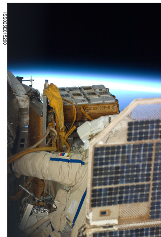
Fig. 4. Installation of EXPOSE-R by EVA at the URM-D platform of the Zvezda module of the ISS. Tray 1 is on top of the picture, compartments 1 are on the right side, and compartments 4 on the left side.
