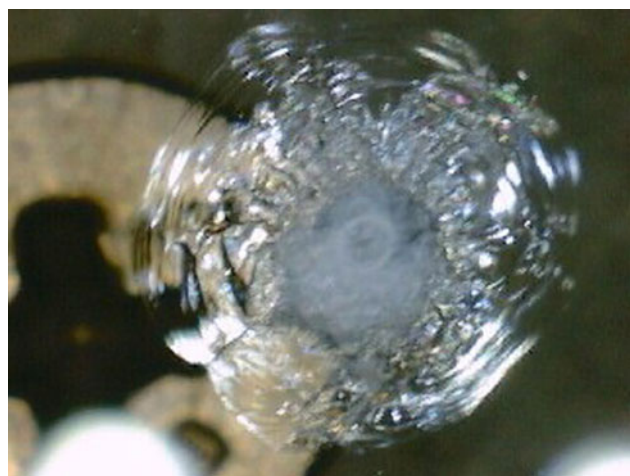
Fig. 6. Micrometeorite impact in the quartz top window of tray 2, compartment 2. Approximate diameter of the fracture: 4 mm (Credit RUAG).
