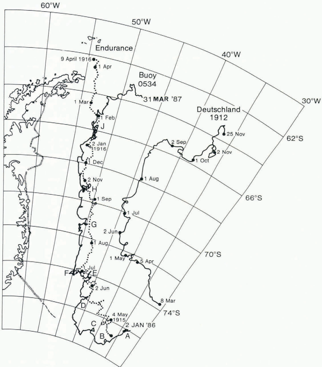
Fig. 1. Tracks of buoy 0534 (from 2 January 1986 to 31 March 1987), of Endurance (1915–16), and Deutschland (1912) (after Ackley, 1979). The letters indicate periods of buoy movement discussed in the text and in Table I.
