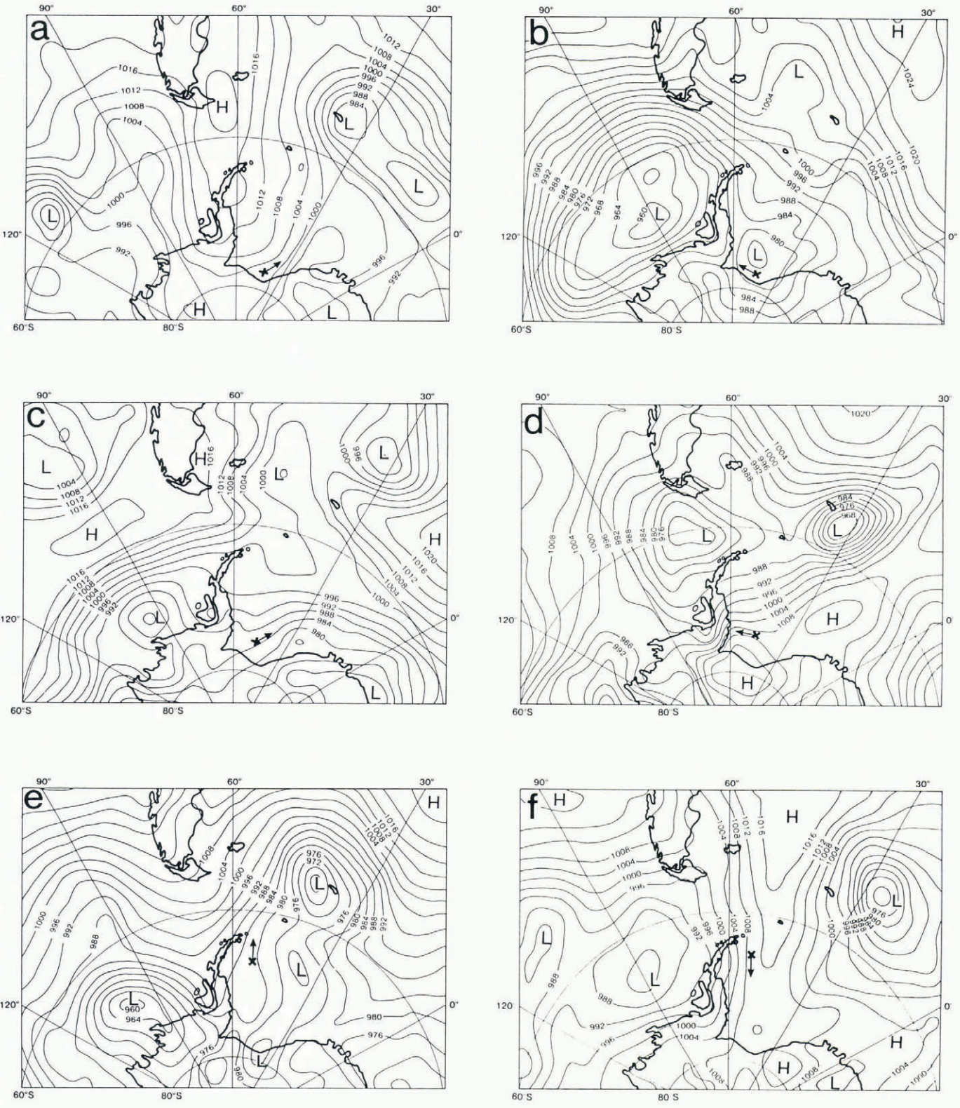
Fig. 2. Surface-pressure charts redrawn from the U.K. Meteorological Office numerical analyses. The approximate position of buoy 0534 and its direction of movement are shown on each by a cross and arrow. The charts are for 00.00 GMT on: (a) 3 March 1986; (b) 11 March 1986; (c) 1 June 1986; (d) 16 June 1986; (e) 31 December 1986; (f) 20 January 1987.
