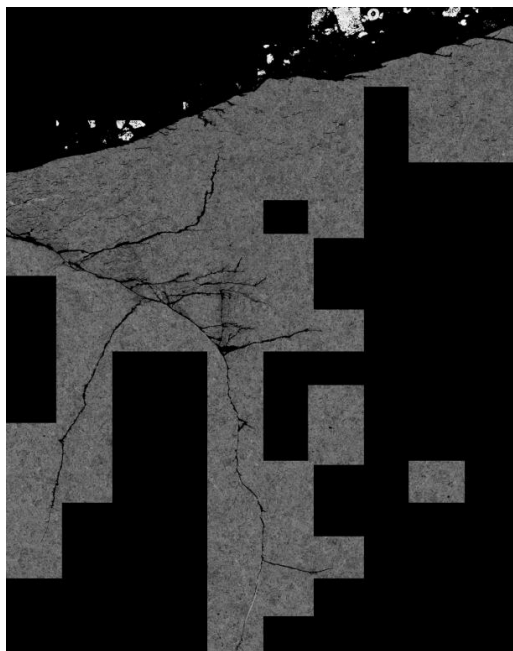
Figure 1: Result of the automated acquisition of high resolution images along the cracks.
