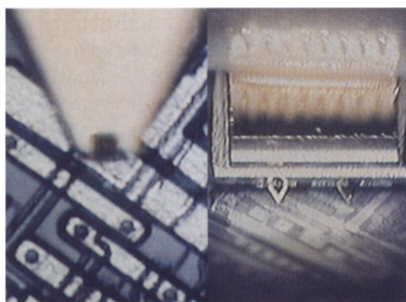
The highest-power, motorized-zoom, color-video, optical microscope system provides on-axis and oblique viewing with a field-of-view from 6mm to 80 \mu m.
