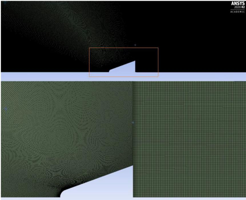
Figure 3. Mesh generated for  $\Delta = 70^\circ$  configuration.
