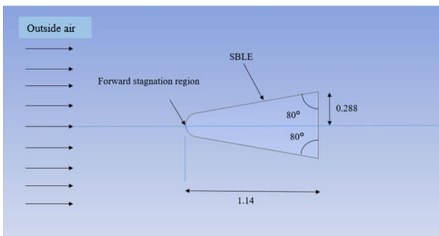
Figure 2. Schematic of the hypersonic vehicle based on  $\Lambda_{HT-min}$ .
