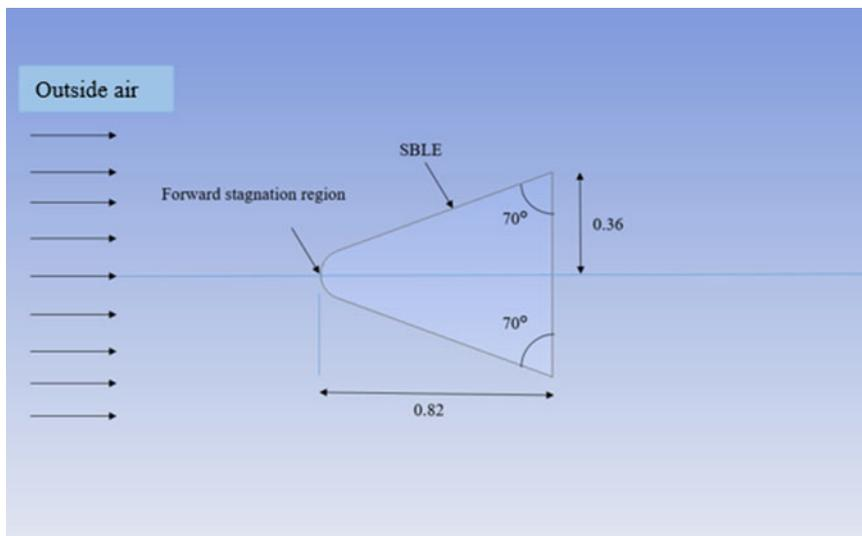
Figure 1. Schematic of hypersonic vehicle based on  $\Lambda_{Drag-min}$ .
