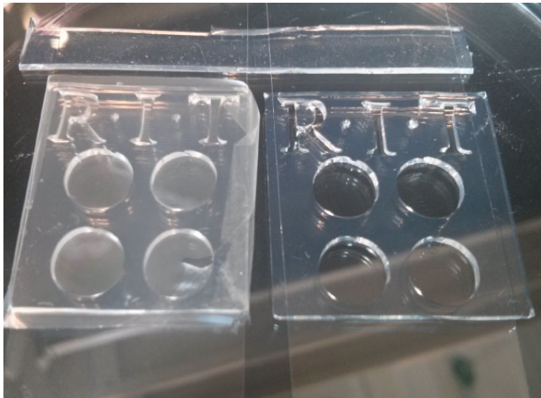
FIG. 1. 50 nm thick microporous silicon nitride with a polymeric scaffold has been lifted off from its silicon wafer substrate. The membrane has been transferred to silicone microwells on a glass slide that span more than 1 square cm.
