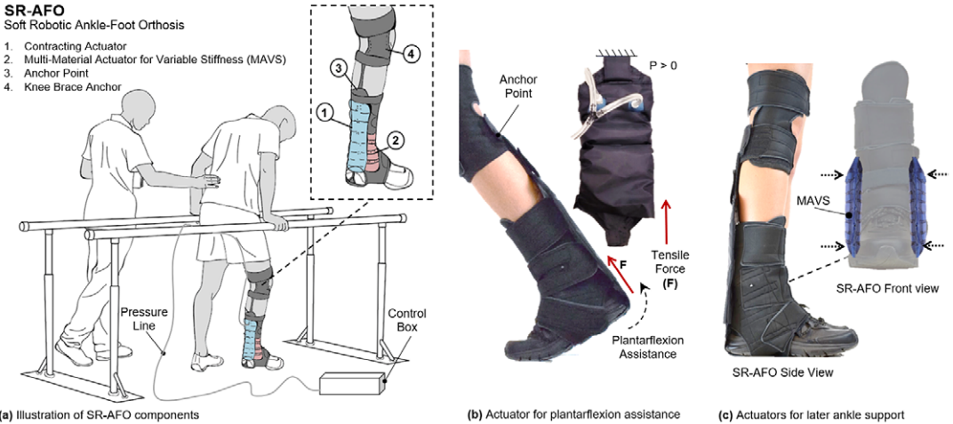
Figure 1. (a) The concept illustration of a soft robotic ankle-foot orthosis (SR-AFO) that assists walking with active ankle plantarflexion assistance as well as medial/lateral ankle support. Since the SR-AFO is designed to be used in its current stages as a rehabilitative device in clinical trials, the goal is to have the participant in a rehabilitative space already equipped with pressure lines, and the hardware needed to control pressure, timing, and record data from each session will sit beside the participant. Ideally, in most cases, there would be no compressor in this setup, rather the electropneumatic hardware box would connect directly to line pressure from the wall. (b) The actuators used for plantarflexion assistance are placed on the back of the leg, and contract to pull the heel upward. (c) The actuators to provide lateral ankle support are placed on either side of the ankle joint, and act as a brace when active to provide variable stiffness to the joint.
