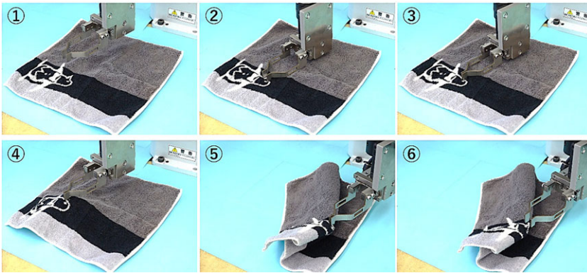
Figure 11. Grasping test of a handkerchief.
