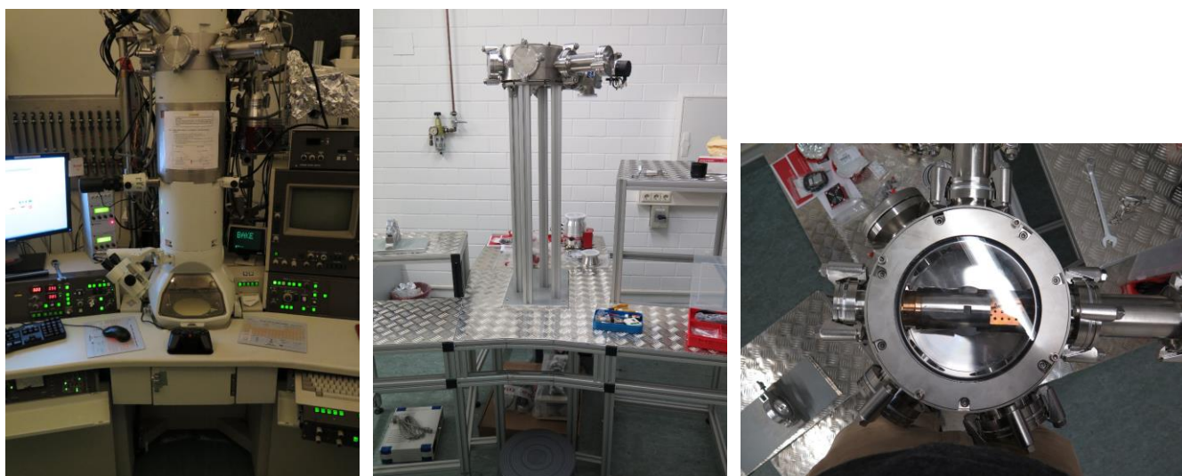
Figure 1. Microscope with new sample chamber, test rack with sample chamber, and sample chamber on test rack viewed along electron beam direction
