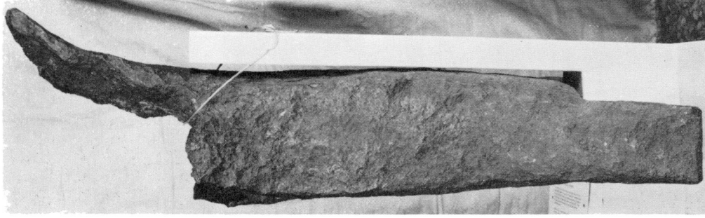
(B) Side view with the casting bent outwards at the break.
