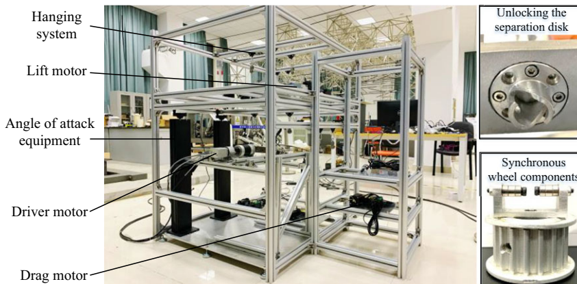
Figure 12. Pneumatic load simulation test platform.
