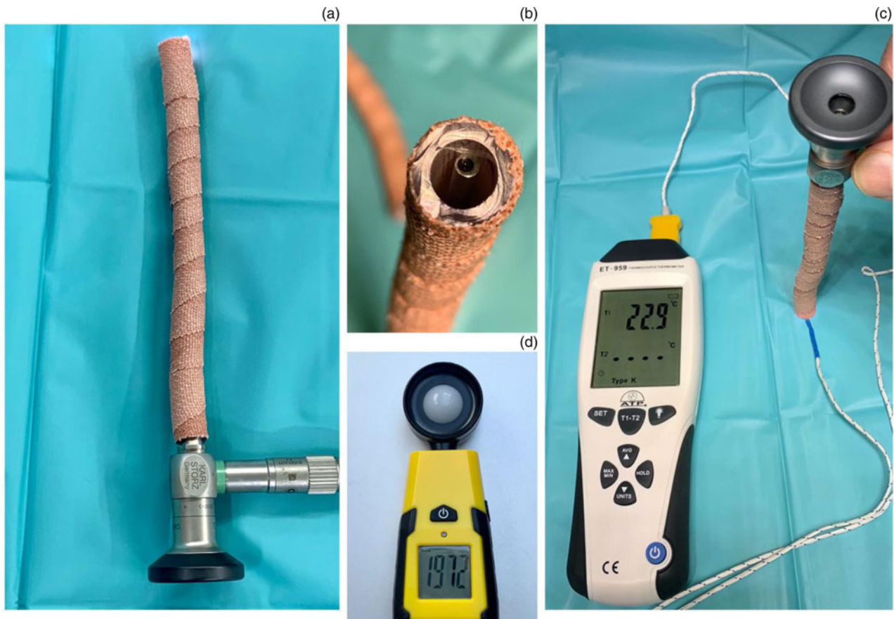
Fig. 1. (a) The set up used to simulate transcanal endoscopic ear surgery using a 7 mm plastic suction tubing, coated in insulating tape, to simulate an external ear canal. (b) The end showing the endoscope tip 5 mm away from the end of tubing. (c) Temperature measurement technique. (d) The luminometer used in the study.
