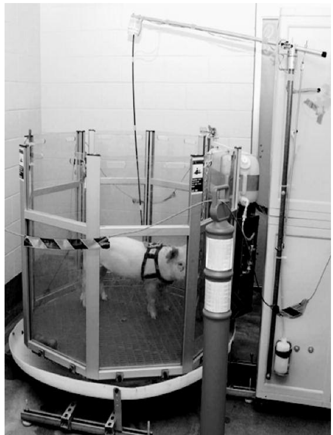
The PigTurn® housing system showing a catheterised pig wearing the harness housed within the octagonal pen, the tether attached to the optical sensor arm and the cabinet unit.
