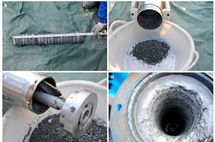
Fig. 8. Tests of the shortened version of the IBED at the outdoor testing stand in debris-containing ice: (a) core with ice/rock mixture layers; (b, c) recovery of chips from the chip chamber; (d) borehole drilled in the sample.
