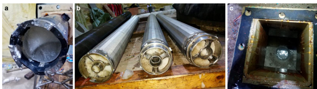
Fig. 6. Tests of the full-scale version of the IBED in an ice well: (a) core barrel with the recovered ice core; (b) chip chambers; (c) ice hole after coring.
