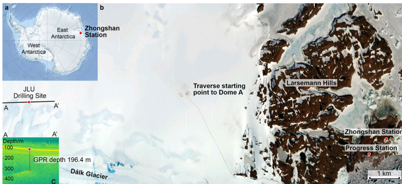
Fig. 10. Drilling-operation area: (a) map of Antarctica, showing the location of Zhongshan Station; (b) Google Map satellite image of the area near Zhongshan Station; (c) ground-penetrating radar profile through JLU drilling site obtained via 'Snow Eagle' airborne radar servicing.
