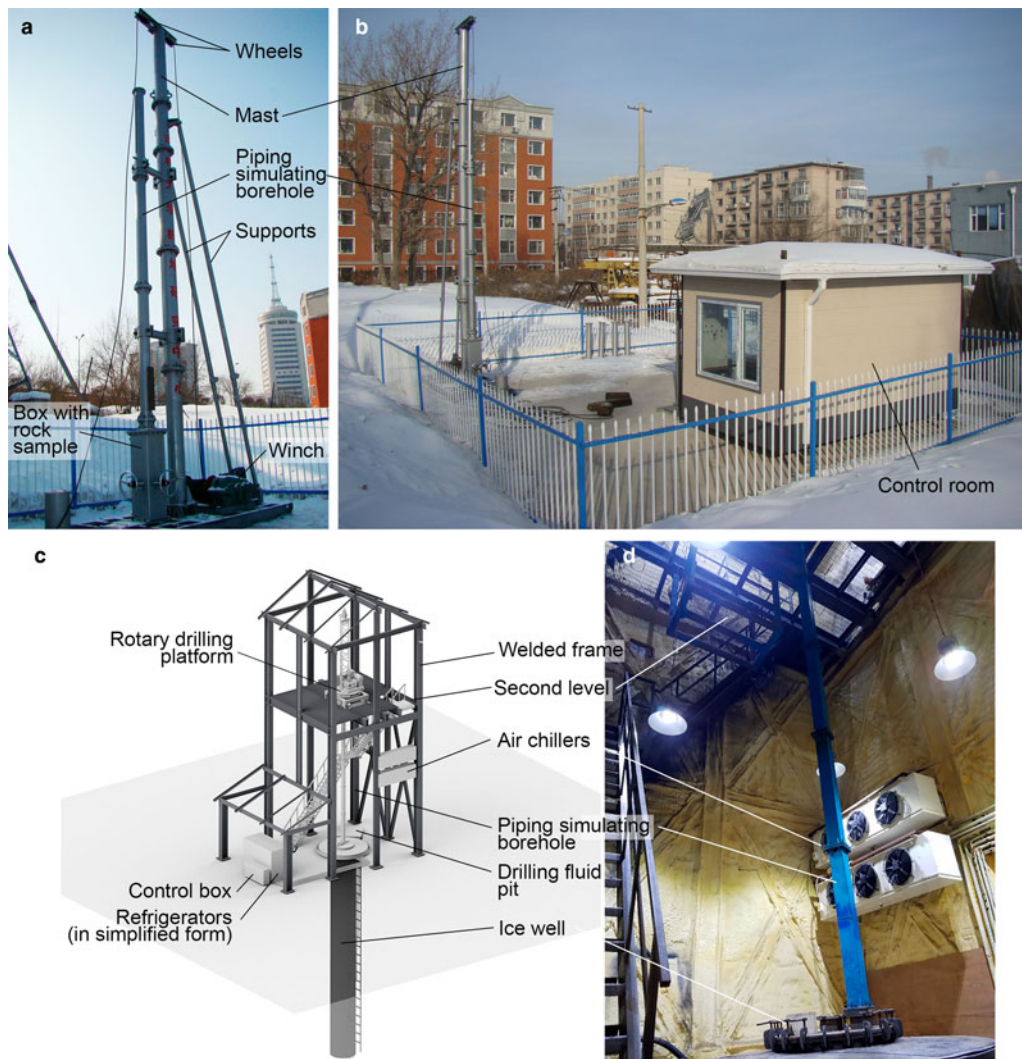
Fig. 3. IBED testing facilities: (a) outdoor testing stand (shortened version of IBED was placed inside piping simulating borehole); (b) outdoor testing site at the Polar Research Center, JLU, Changchun; (c) general structure of the ice-drill testing facility with a 12.5 m-deep ice well; (d) view inside the tall hall of the ice-drill testing facility with square steel piping simulating the borehole.
