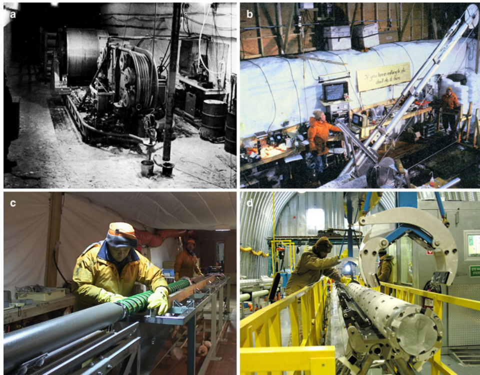
Fig. 1. Examples of electromechanical cable-suspended drills: (a) electrohydraulic hoist with 3650 m of cable and CRREL drill in the foreground, Byrd Station, West Antarctica, 1967–1968 season; (b) drilling operations with ISTUK drill at Dye-3, Greenland, 1981; (c) JARE drill in Dome F drilling trench, East Antarctica, season 2005–2006; (d) DISC drill servicing, WAIS Divide, West Antarctica, 2007–2008 season (all photos from Talalay, 2016).
