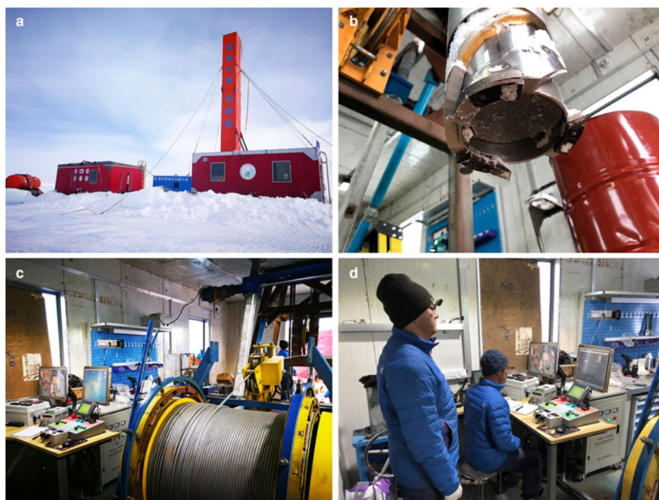
Fig. 11. Drilling operations at the JLU drilling site in the vicinity of Zhongshan Station, East Antarctica: (a) drilling camp; (b) auger version of the IBED with the ice core; (c) drilling winch and control desk; (d) drilling process monitoring.
