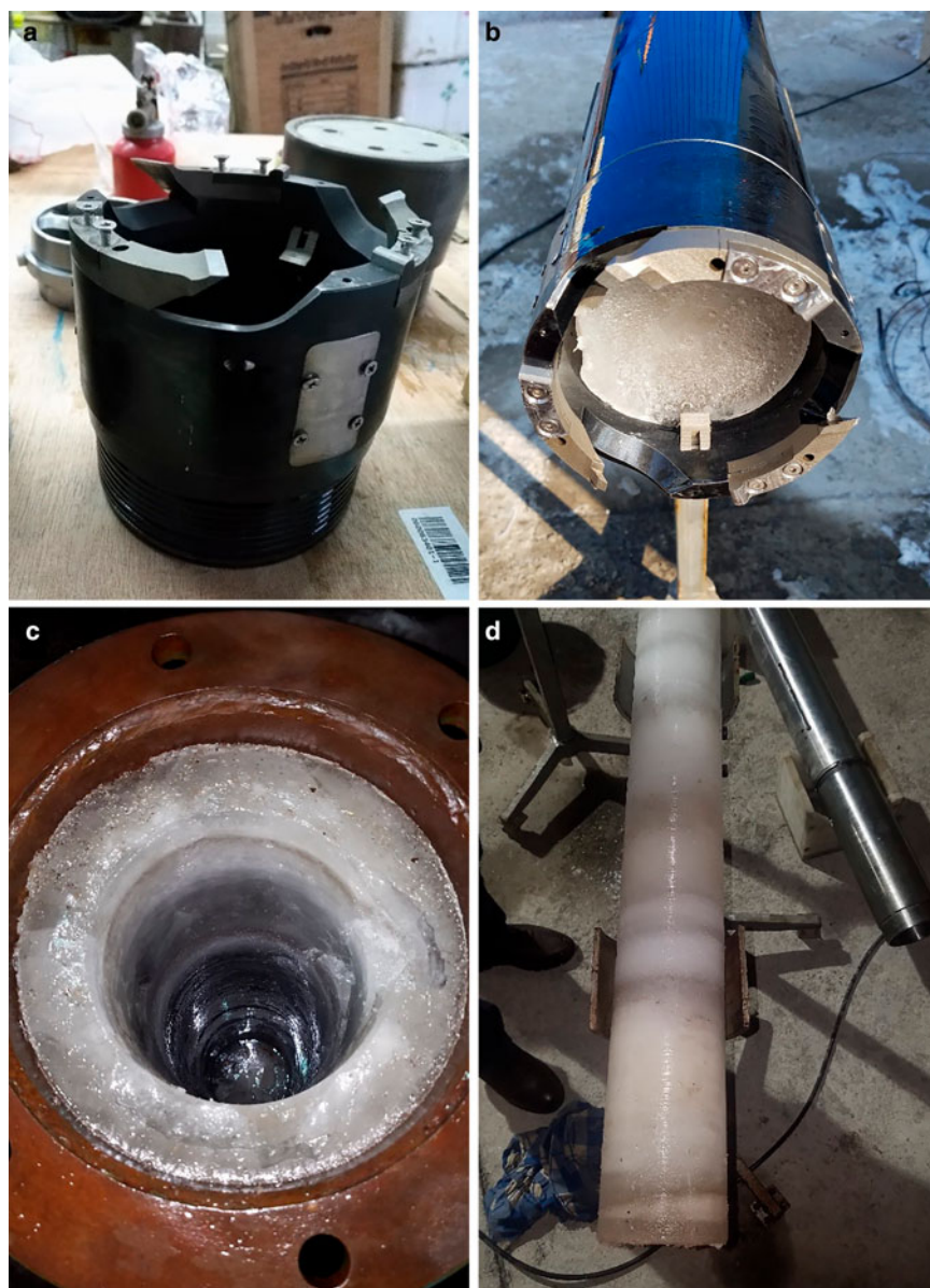
Fig. 4. Ice-drilling tests of the shortened version of the IBED at the outdoor testing stand: (a) ice-drill head; (b) core barrel with the ice core; (c) borehole drilled in an ice sample; (d) recovered ice core.
