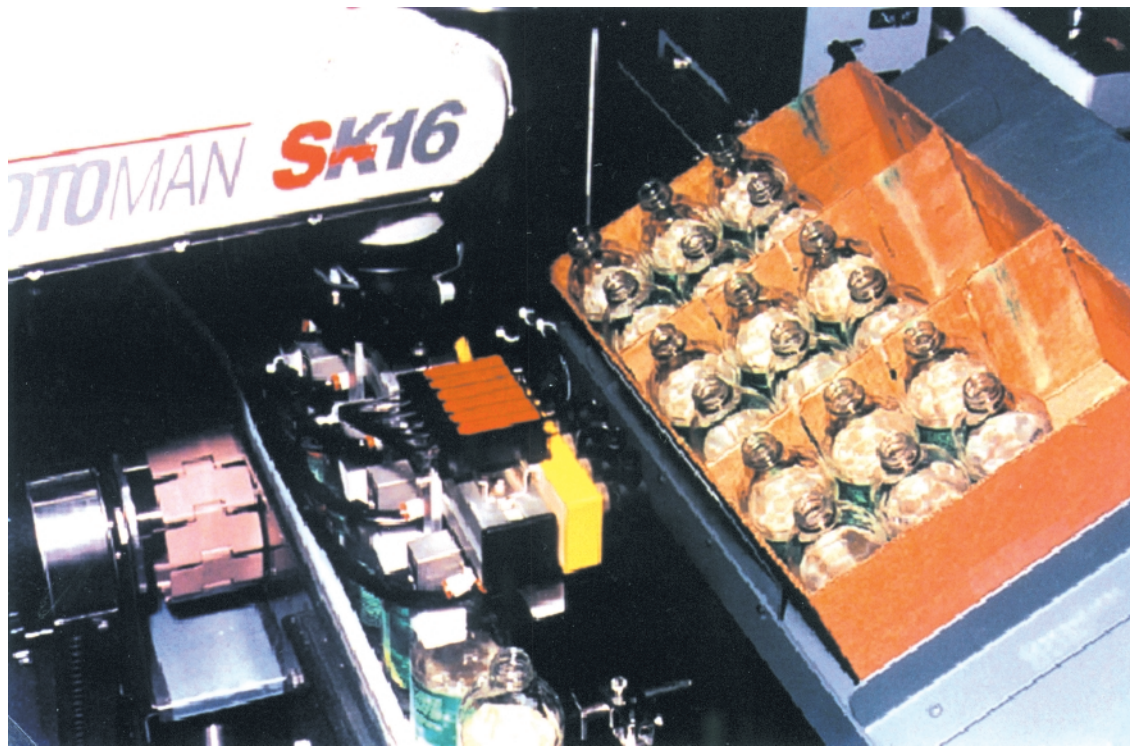
Fig. 1. Close-up of a Motoman robot packing bottles in an automated handling cell of the type exhibited at the BPC 2000.
