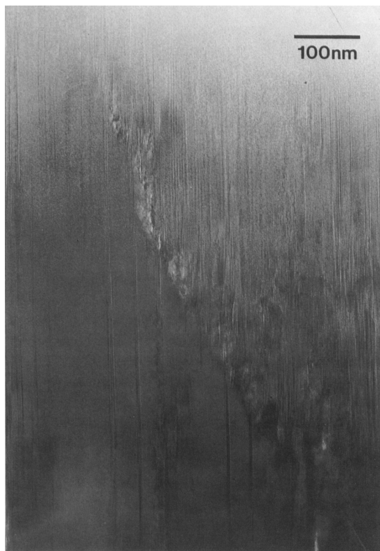
Figure 5. Transmission electron micrograph of a chlorite grain in sample KC-813, illustrating a high-strain zone with abundant layer distortions cutting across the cleavage. Stacking faults (linear contrast features) are abundant on both sides of the high-strain zone.
