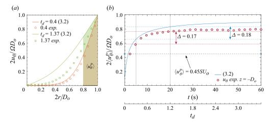
Figure 12. (a) Comparison between  $u_{\theta}$  profiles from experiments measured at  $z = -D_o$ ,  $\Omega = 1.95$  rad s<sup>-1</sup> (S = 1) and that based on (3.2), at  $t_d = 0.34$  (t = 6 s) and 1.36 (24 s). The shaded area represents  $\langle u_{\theta}^p \rangle$  averaged over  $0.4 \leq r/D_o \leq 0.5$  according to (3.20). (b) The evolution of  $\langle u_{\theta}^p \rangle$  in physical preparation time; the second abscissa is the corresponding diffusion time  $t_d$ .
