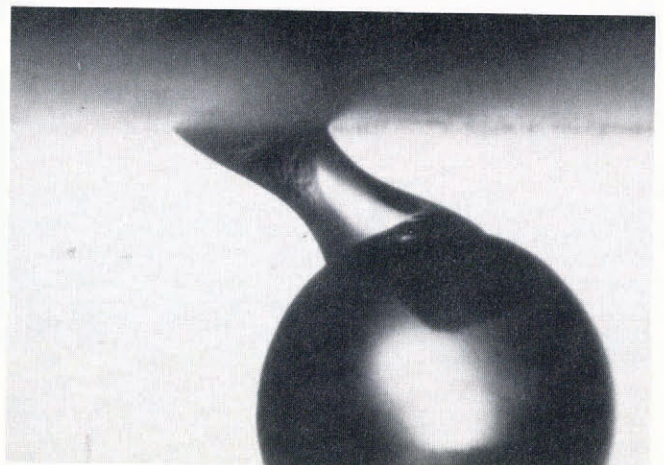
Fig. 4. Water held between a hydrophilic bead and a teflon slider while the slider is moving to the left. This water bridge would exert a drag on the slider without supporting any weight.
