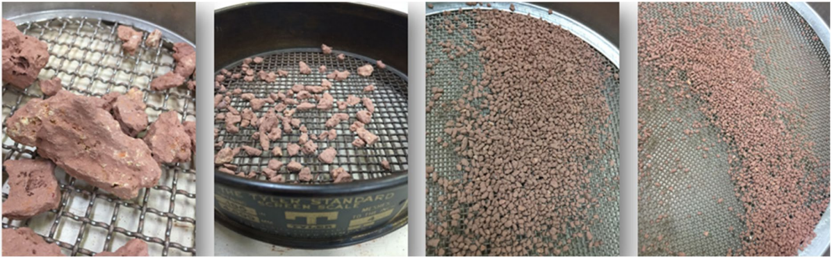
Fig. 3 Bauxite sample during grain-size distribution tests
