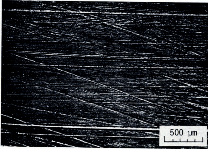
Fig. 3. Photomicrograph showing the ice surface treated with an emery paper.
