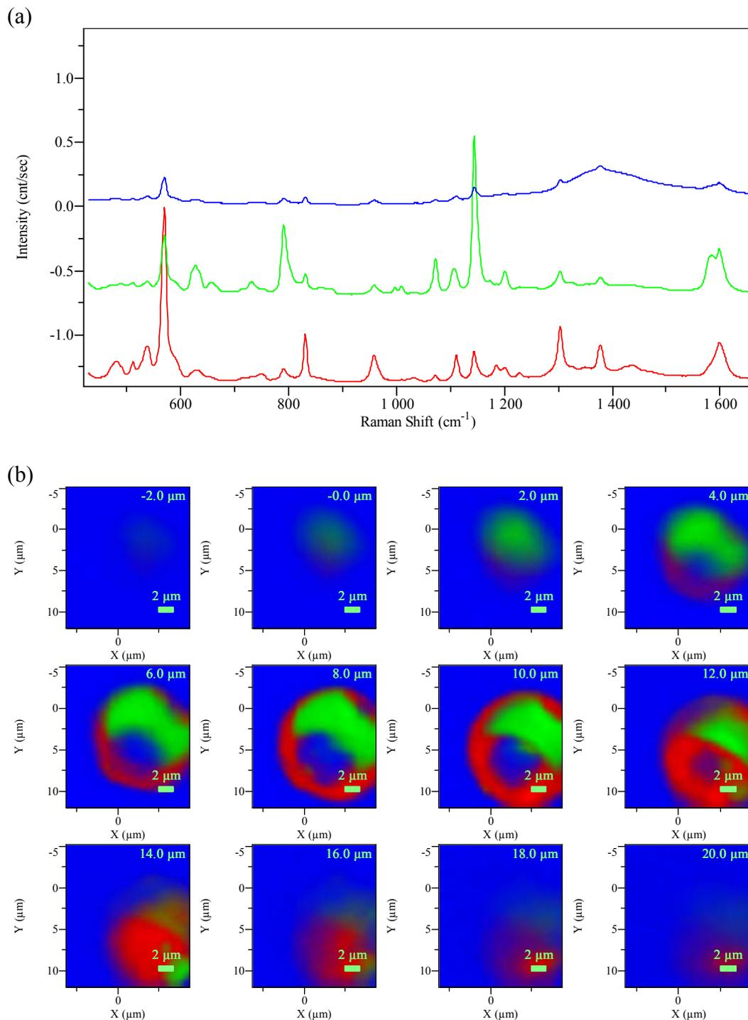
Figure 1. Confocal Raman hyperspectral imaging results from a thermoplastic bead, processed by direct classic least square regression. (a) Models that are statistically representative of spectral species present and (b) score images (color-coded to models) that represent the spatial distribution of identified spectral species. Numbers marked in each score image is the relative height of the sample.
