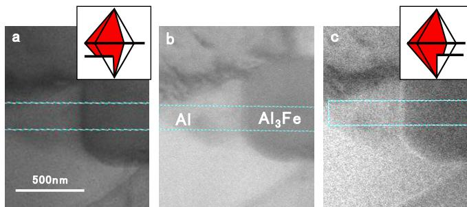
**Figure 3.** BF image of the interface with the aperture in (a) right, (b) without, (c) left hand side, and corresponding intensity profiles (d), (e) and (f), respectively. Insets are the schematic drawing of geometrical optics of the deflected beam with the aperture.
