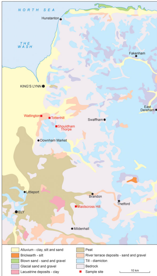
Fig. 2. Quaternary geological map of the study region, showing the glacial deposits, gravel spreads and the Fenland Holocene deposits. The approximate ‘Skerterchly Line’ glacial maximum limit is also shown. Map source: EDINA.
