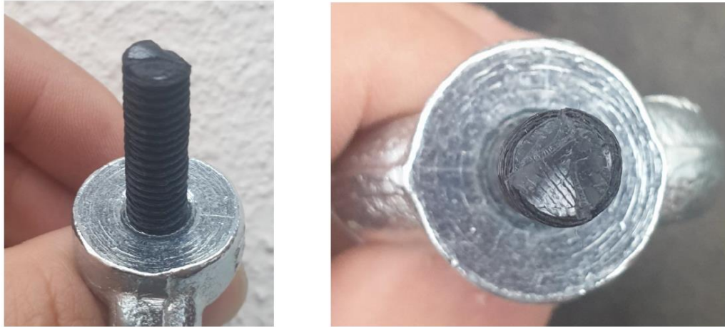
Figure 7: Failure pattern of a tensile specimen
