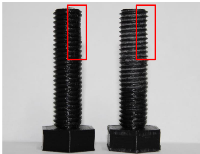
Figure 5: Comparison of pre-damaged specimen (left) and resulting re-rolled thread (right)
