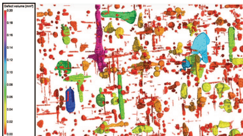
Figure 4: Image of the volume size distribution of pores in a carbon-epoxy composite. The width of the image to scale is 13.8 mm.
