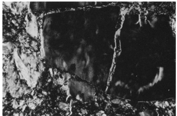
Figure 3. Photomicrographs of sample OU 45968 from the Acheron debris flow. Upper = veins of cross-fiber chrysotile (light-colored) cross-cut and cement breccia clasts (dark). Opaque minerals are magnetite (in clasts) and a Ti-oxide (in clasts and veins). Plane polarized light; horizontal field of view = 2.4 mm. Lower = fractured lizardite clast (dark) which has been coated and veined by slip-fiber and cross-fiber chrysotile (white rim on clast fragments). Crossed polars; horizontal field of view = 4 mm.
