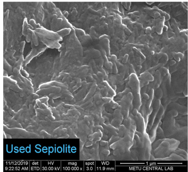
Fig. 4. SEM images of the sepiolite samples.
