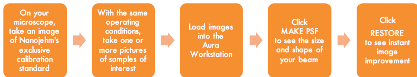
Figure 2: Flow diagram showing the determination of the PSF and the image restoration process.
