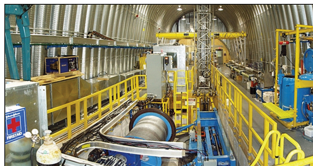
Fig. 2. DISC drill system layout at WAIS Divide.
