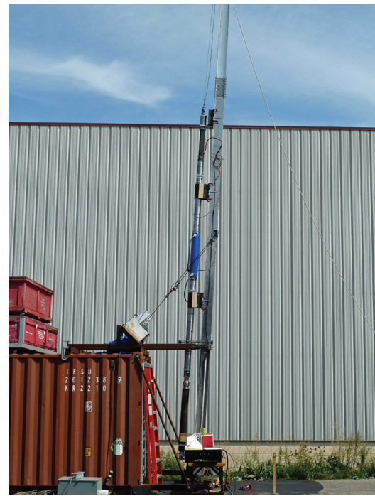
Fig. 22. Drill deflection simulator.
