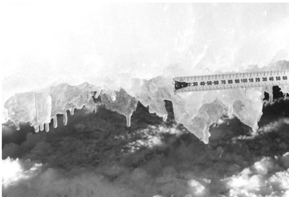
Fig. 2. Base of sea-ice slab taken at CH site, showing attached platelet ice.
